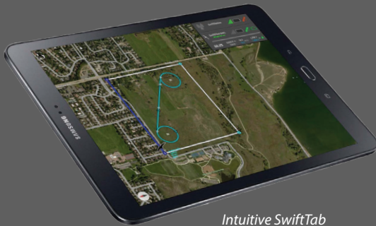
Intuitive SwiftTab user interface controls all autopilot, mission and aircraft parameters.
